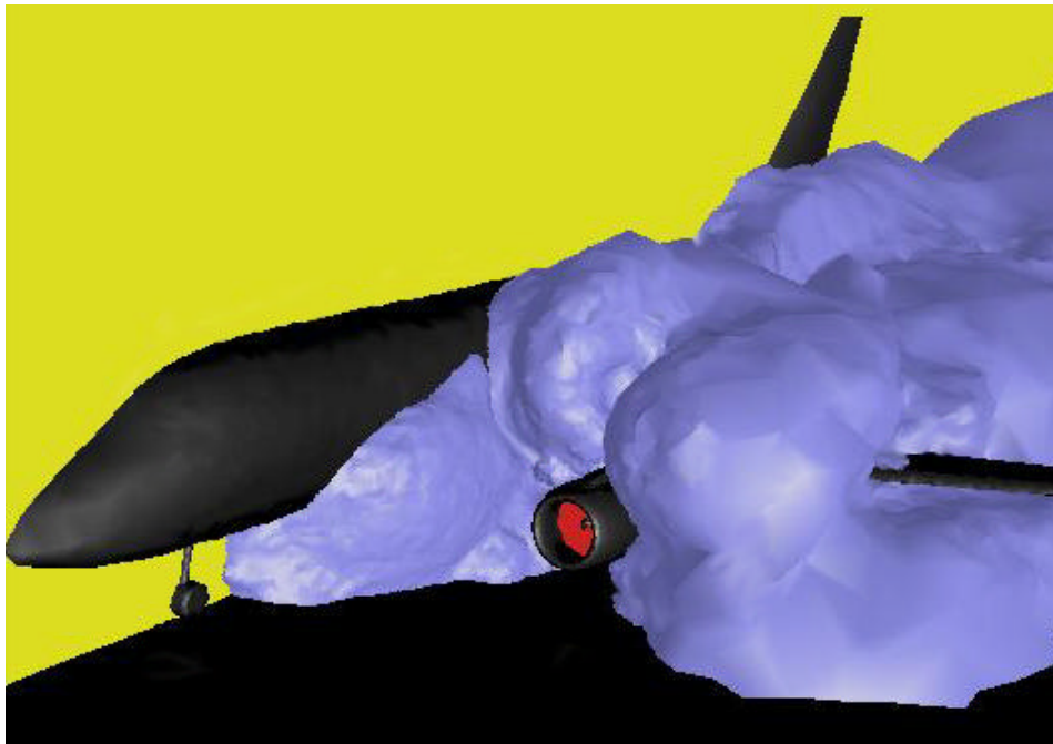
Figure 5. Thrust reverser plume - isosurface of total temperature.
