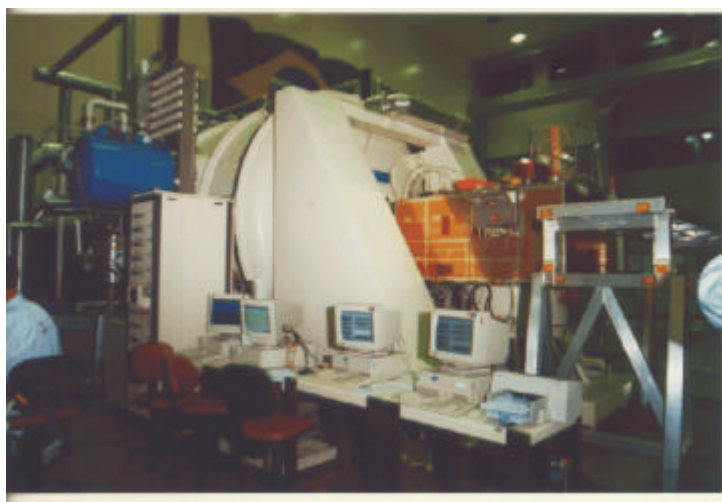
Figure 6. SM Space Simulation - view of the setup involved including the T/V Chamber, with the PM positioned outside and connected by cables to the SM, by its turn installed inside the chamber.
