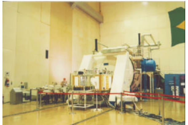
Figure 12. Left: PM installation in the 3m x 3m T/V Chamber. Right: view of the complete setup, including the SM positioned outside the T/V Chamber (which was connected by electrical cables to the PM installed inside the chamber)
