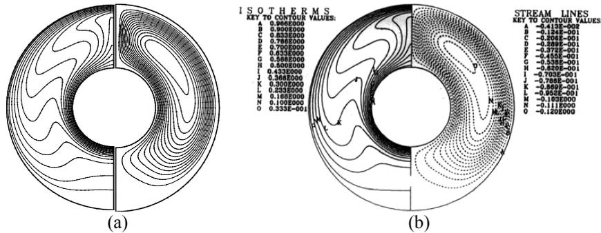
Figure 3. (a): Isotherms and Streamlines for a laminar flow in a concentric annulus with  $Ra_L=5 \times 10^4$ ,  $R_i/R_o=0.3846$ , (b): Kenjeres & Hanjalic, (1995)
