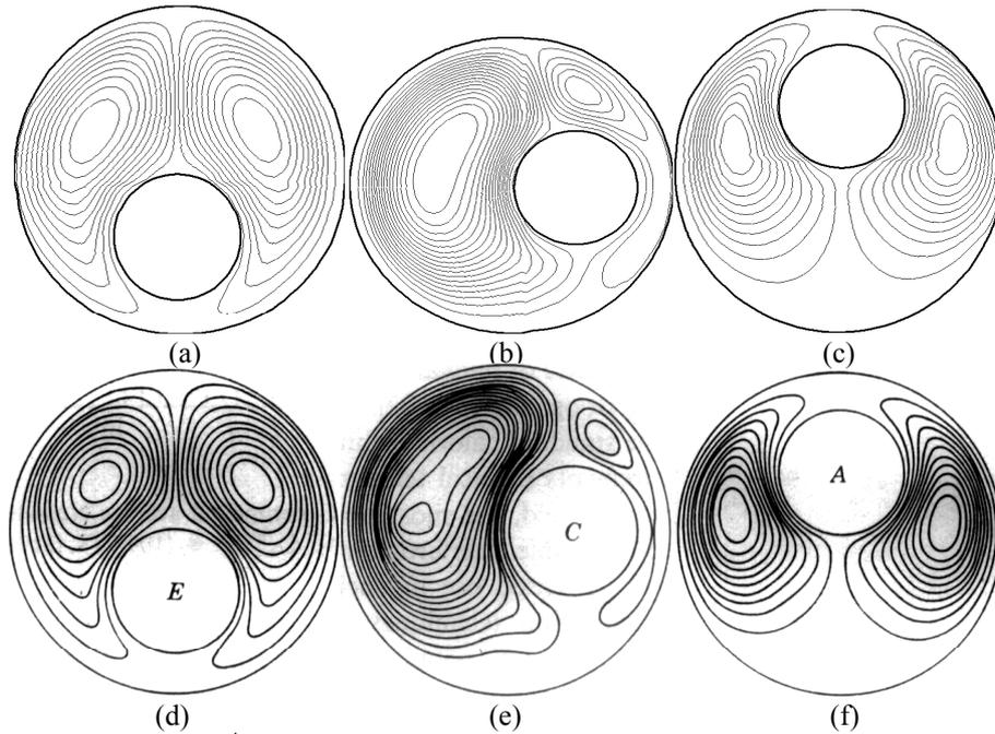
Figure 5. Streamlines for  $(Ra_L=10^4, R_i/R_o=0.3846, e=0.623)$ , Present Results, (a), (b) and (c), Cho et al, (1982), (d), (e) and (f)
