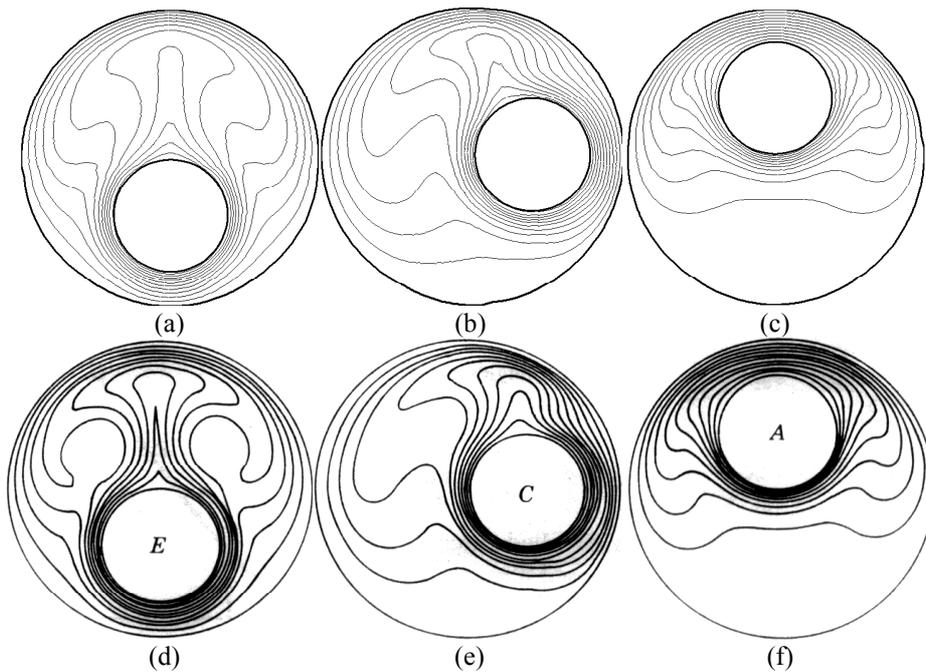
Figure 6. Isotherms for  $Ra_L=10^4, R_i/R_o=0.3846, e=0.623$ . Present Results, (a), (b) and (c); Cho et al, (1982), (d), (e) and (f).
