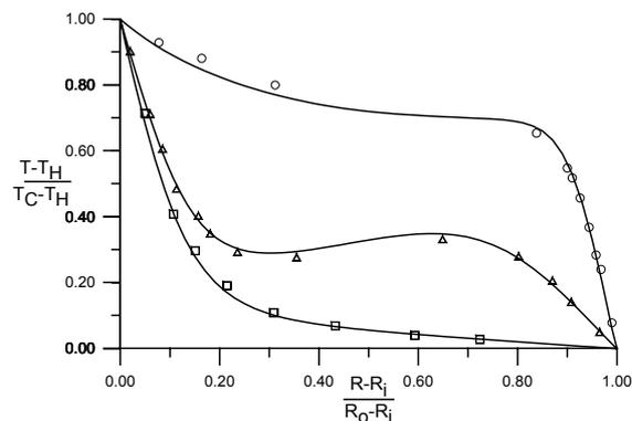
Figure 4. Temperature behavior for laminar regime in a concentric annulus,  $R_i/R_o=0.3846$ ,  $Ra_L=5 \times 10^4$ , Symbols: experiments of Kuehn & Goldstein, (1978),  $O \Rightarrow \theta=0^\circ$ ,  $\Delta \Rightarrow \theta=90^\circ$ ,  $\square \Rightarrow \theta=180^\circ$
