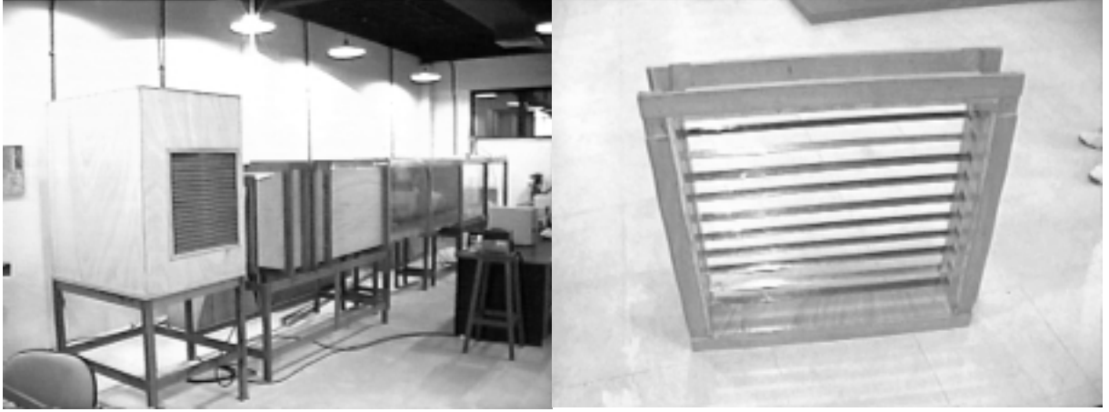
Figure 1. General view of wind tunnel and the heating elements.
