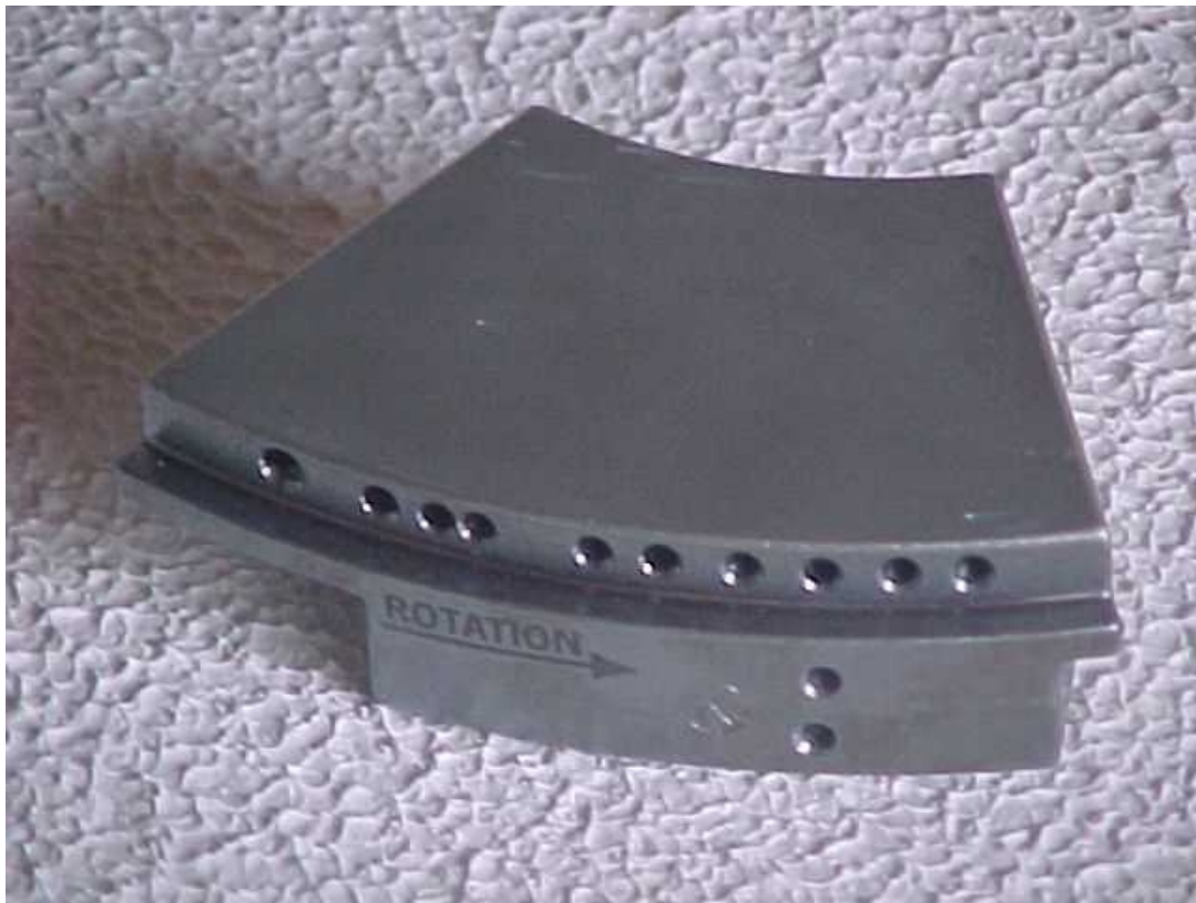
Figure 5. A 66% pivoted pad, prepared for thermocouple insertions.
