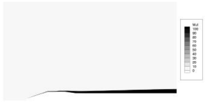
Figure 6: Turbulent viscosity contours for the case with Liou's second order scheme and the Spalart and Allmaras model ( M_{\infty} = 0.90 and Re = 20 \times 10^6 ).
