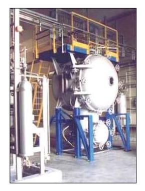
Specially designed and built to attend the needs of the Brazilian Space Program, INPE's Test Bench with Altitude Simulation, in Cachoeira Paulista, Brazil, is one of the most sophisticated instruments in the qualification of satellite thrusters, with its convenient eight cubic meters chamber.
