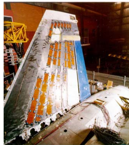
Figure 3 – F-18 instrumented vertical fin.
