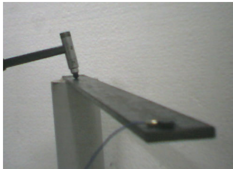
(b) beam structure, impact hammer in first position and accelerometer.
