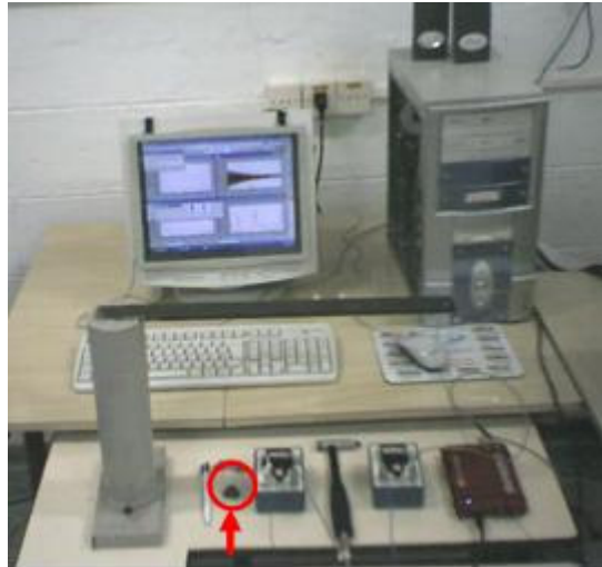
(a) Beam structure and experimental setup; the additional mass = 16g is shown in the circle.
