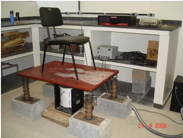
Figure 1. A Picture of the WBV Test Platform.
