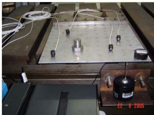
Figure 4 - Localization of the two masses added on the aluminum plate for the accomplishment of the tests.
