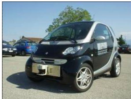
Figure 3 – Modified Smart Car used at ASL. Observe the LMS 291 SICK laser sensor assembled on its front bumper.
