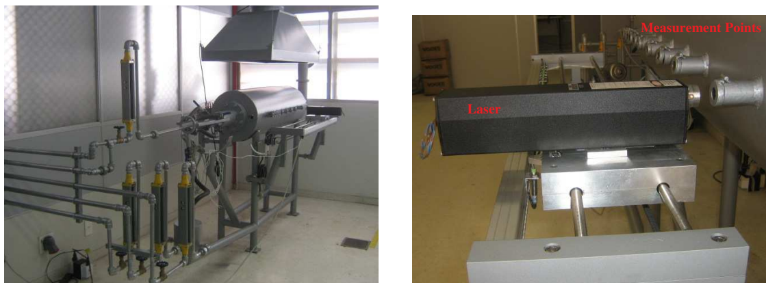
(a) View of Combustion Chamber and Rotameters. (b) View of laser system and ten points for soot measurement.
