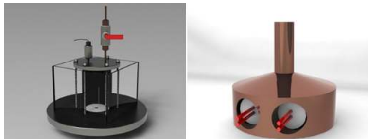
Figure 2 – Transparent boiling chamber and, in detail, the heating section without Teflon cover
