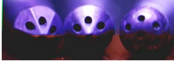
Figure 3. Faceted, conical and hemispherical seven-hole tips
