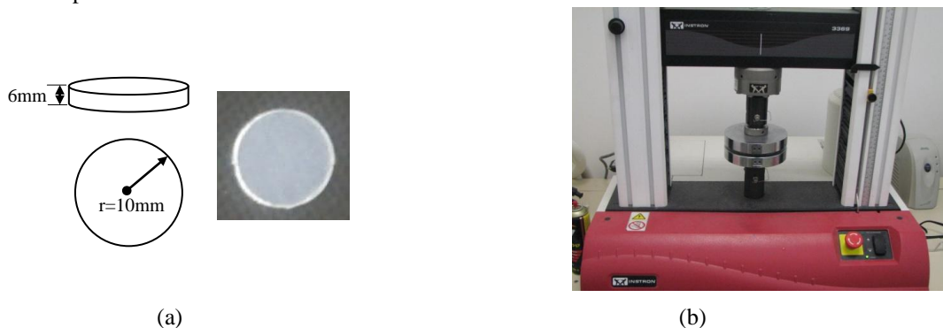
Figure 1. (a) Compression tests specimens and (b) set up and the experimental apparatus.
