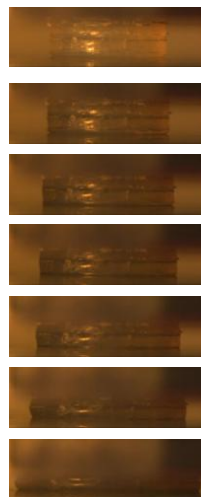
Figure 2. Compression test, recorded by a high velocity camera.
