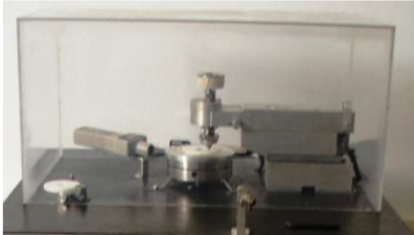
Figure 1 – Pin-on-disc wear testing machine
