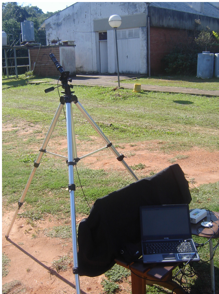
Figure 2. Spectroradiometer EPP2000 and portable computer to measure the spectral cloud transmittance in the Laboratório de Energia Solar of UFRGS (lat. 30.1S, long. 51.1W).
