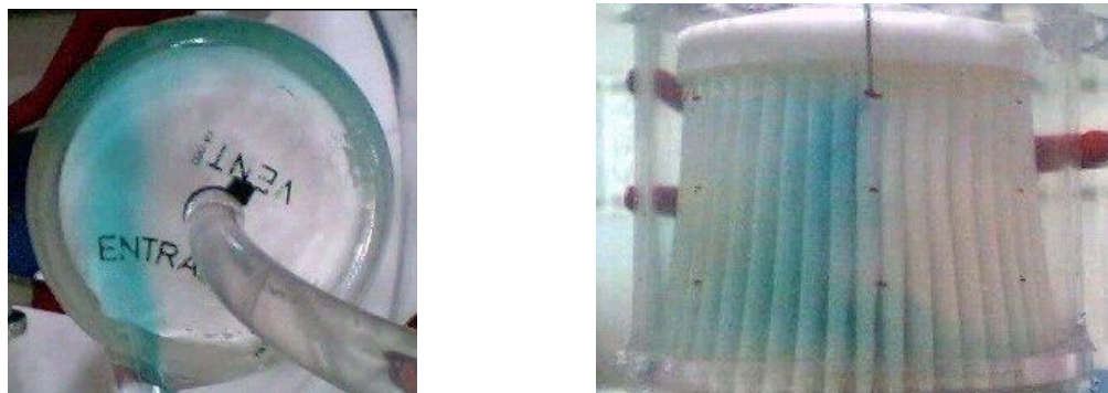
Figure 8. Top view showing the flow direction and the division at the exit connector neighborhood (Huebner, 2003)
