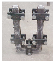
Figure 1 – Split mold in “U” shape
