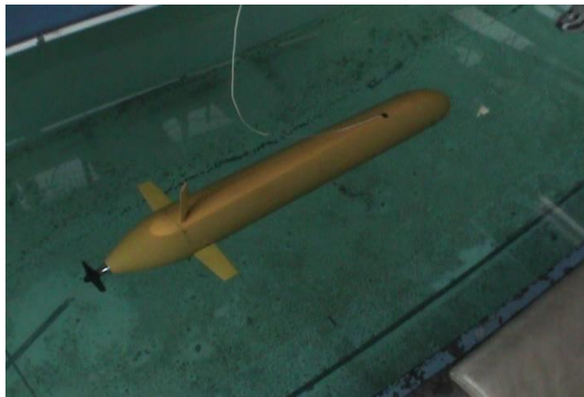
Figure 1. AUV Pirajuba under a self-propelled tank test in the IPT.
