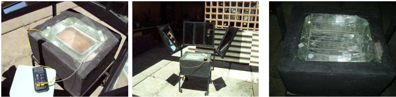
Figure 7. Constructive details of the changes made in solar oven / cooker.
