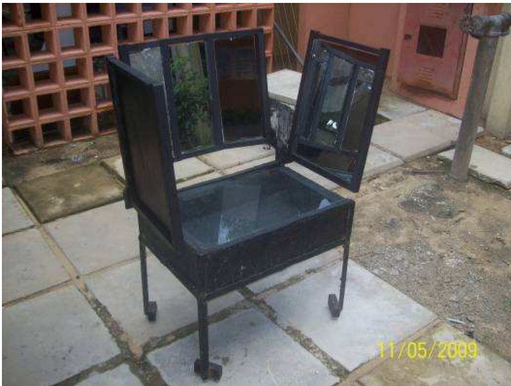
Figure 2. Solar oven/cooker in solar test.
