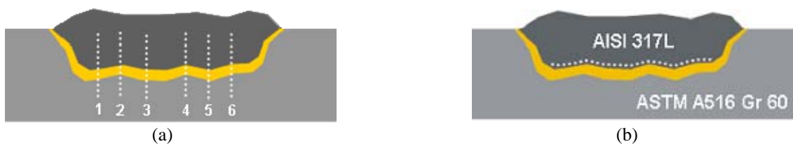
Figure 3. Methodologies for microhardness testing: (a) indentations along the vertical lines (and load of 0.3kg) and (b) indentations along the fusion boundary, inside the WM (load of 0.1kg).
