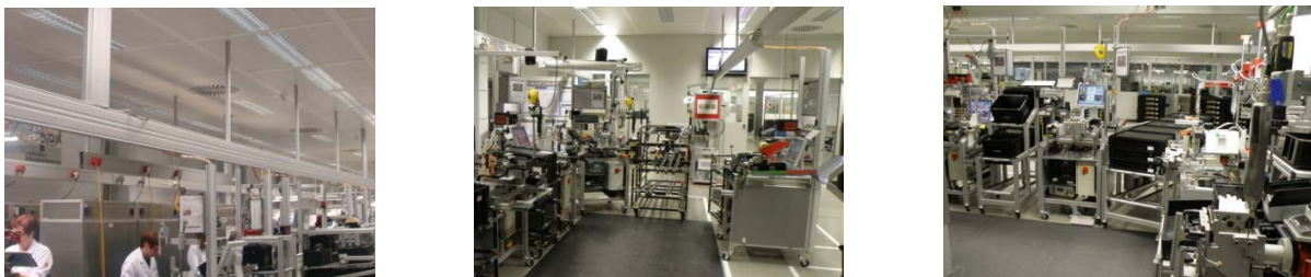
Figure 12 - Example of flexible lines with wheels and pipe conveyors fixed to the ceiling.
