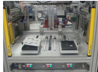
Figure 10 - Robot with three screwing bases.
