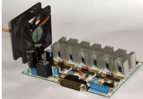
Figure 3. Unipolar stepper motor controller, model SMC-U-V XYZ 1:30
