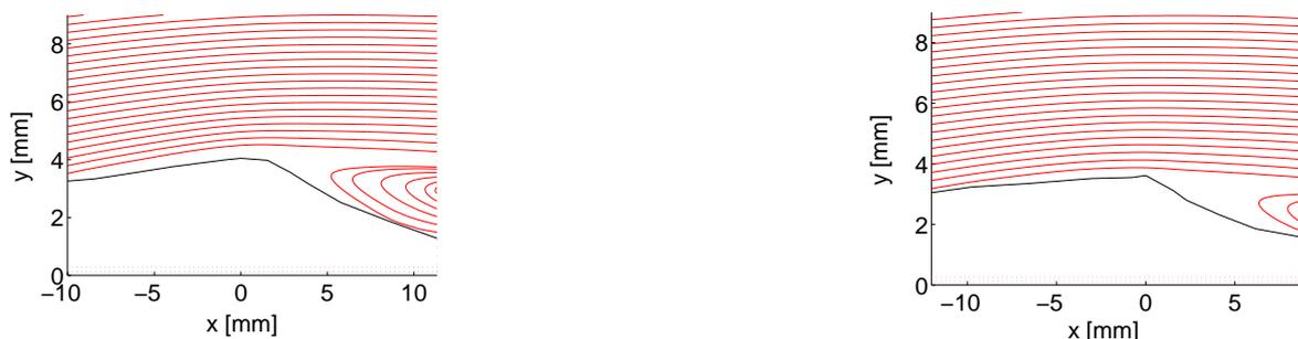
Figure 6. Lower half of the mean velocity field above a barchan dune, in terms of streamlines. In the left,  $Re = 9300$  and there is no bed-load. In the right,  $Re = 13900$  and there is bed-load. Streamlines are shown here with the half of PIV resolution.
