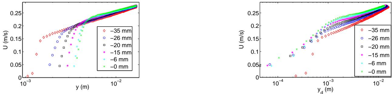
Figure 7. Some profiles of the mean longitudinal velocity over a barchan dune, in semi-logarithmic scale :  $Re = 13900$ . The legend indicates the longitudinal positions where the profiles were taken, 0 being the position of the crest.
