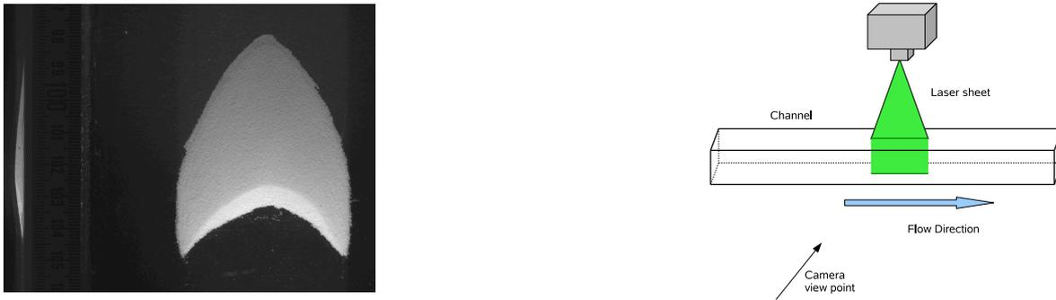
Figure 2. In the left, example of image obtained by the camera/mirror device (on the right we have a direct top view of the barchan dune by the camera and on the left we can see the barchan profile reflected by the mirror and indirectly caught by the camera). The fluid flow is from top to bottom. In the right, PIV experiment layout.
