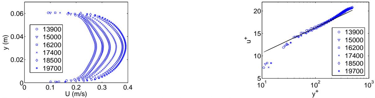
Figure 3. (a) mean longitudinal velocity profile in linear scale. (b) mean longitudinal velocity half-profile in semi-logarithmic scale. Symbols in the figure correspond to  $Re$ .  $y^+ = yu_*/\nu$  and  $u^+ = u/u_*$ .
