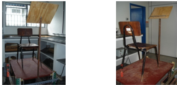
Figure 3. Details of the pedestal and chair used during the reading WBV tests
