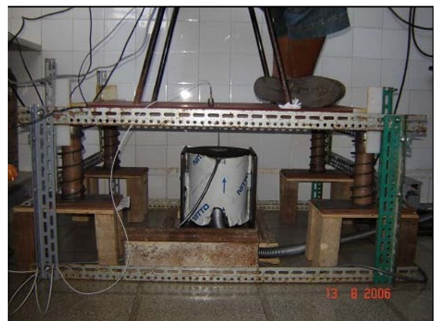
Figure 2. Photo of the setup used for WBV Reading Tests
