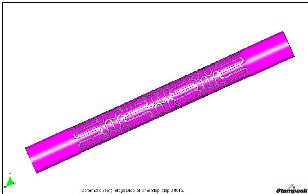
Figure 5 – Stent crimped on the idealized balloon.
