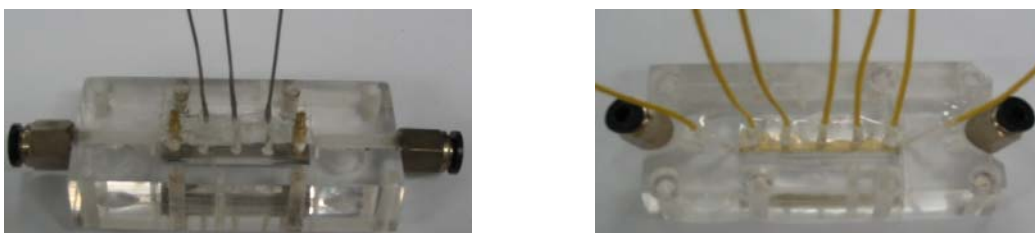
Figure 3 – Details of the lower and upper plates of the microchannel setup with installed thermocouples.
