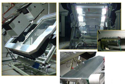
Figure 6. Samples in the test of thermal efficiency in solar simulator.
