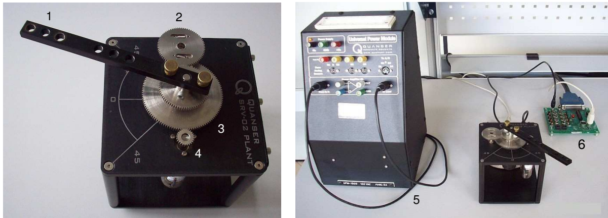
Figure 2. Quanser servo positioning arm platform: 1) arm; 2) potentiometer; 3) main shaft + encoder; 4) electric motor + gear box; 5) power module; 6) acquisition board.
