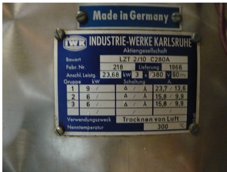
Figure 5. Spray dryer specifications.
