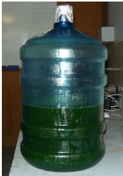
Figure 1. Microalgae after flocculation, settling and packaging in 0.02 \text{m}^3 vessel.
