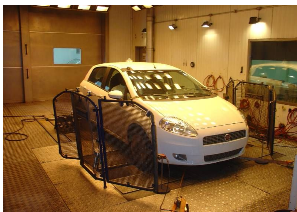
Figure 3. Vehicle mounted in the climate chamber with dynamometer roller.
