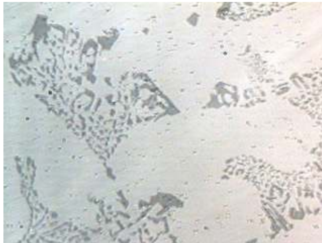
Figure 2. Microstructure of the Al-Si alloy, evidencing the light phase rich in aluminum and eutectic.
