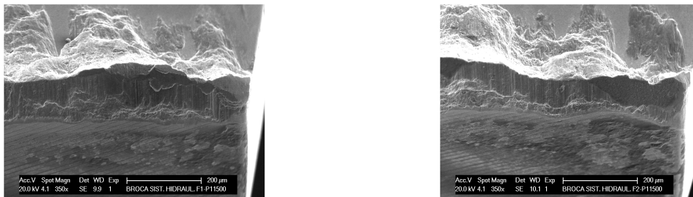
Figure 9. Presence of material parts on drill faces 1 and 2 of the hydraulic system part 11500
