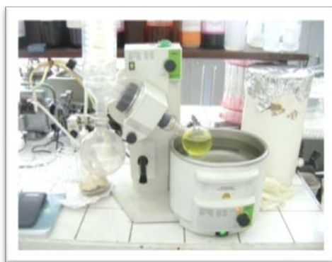
Figure 3. Rotavapor vacuum system
