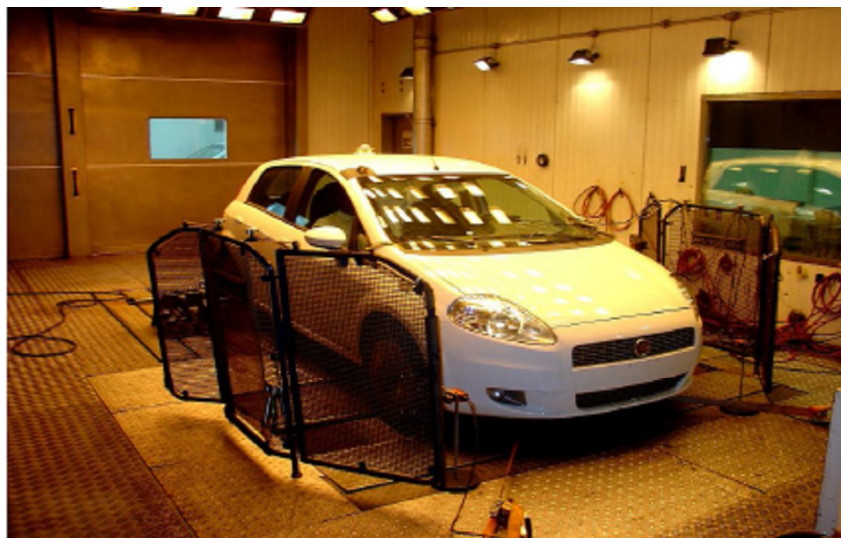
Figure 5. Vehicle tested installed in the roller dynamometer.
