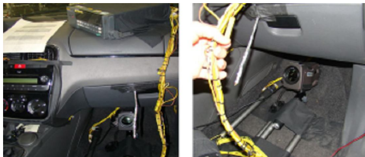
Figure 2. Thermographic camera attached to the passenger compartment inside of vehicle.
