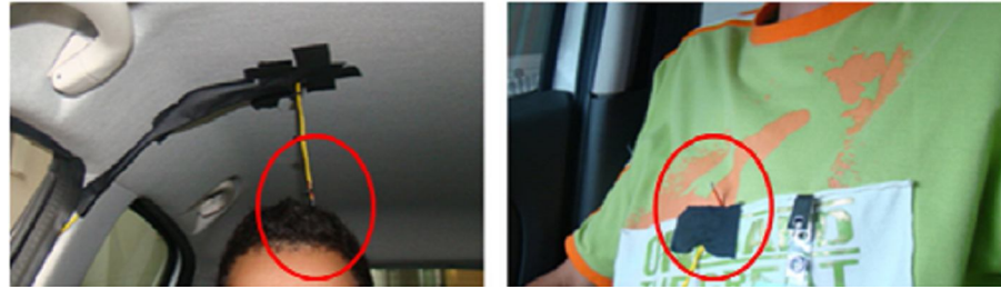
Figure 3. Place of thermocouples installation.
