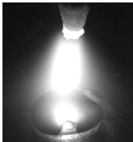
Figure 2. TIG on mild steel 100A, pure Ar.
