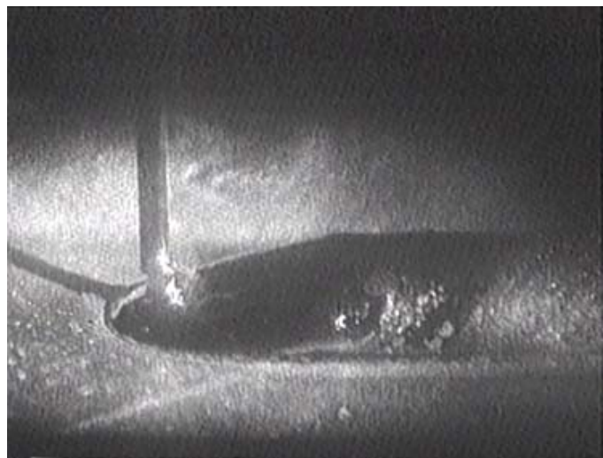
Figure 4. MIG Weld pool images.
