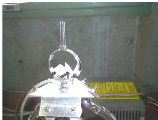
Figure 12 - Force sensor (strain gages attached in a metallic ring linked in Wheatstone bridge).
