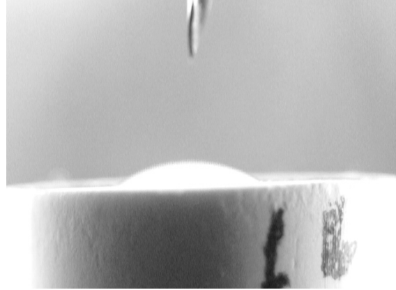
Figure 7. Fast water drop absorption on A-S5G \text{Al}_2\text{O}_3 surface (not treated with plasma).
