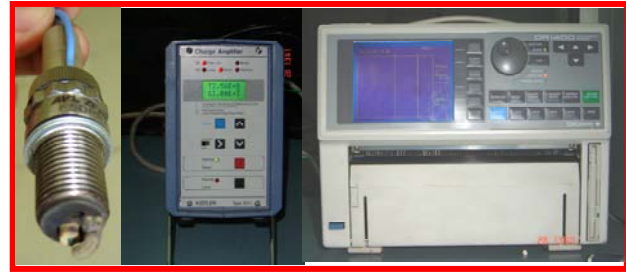
Figure 2 – The Spark plug transducer, charge amplifier oscillographic data logger
