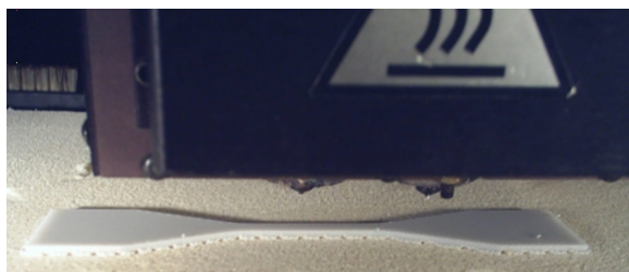
Figure 14. Tensile test specimen being built in the FDM 2000
