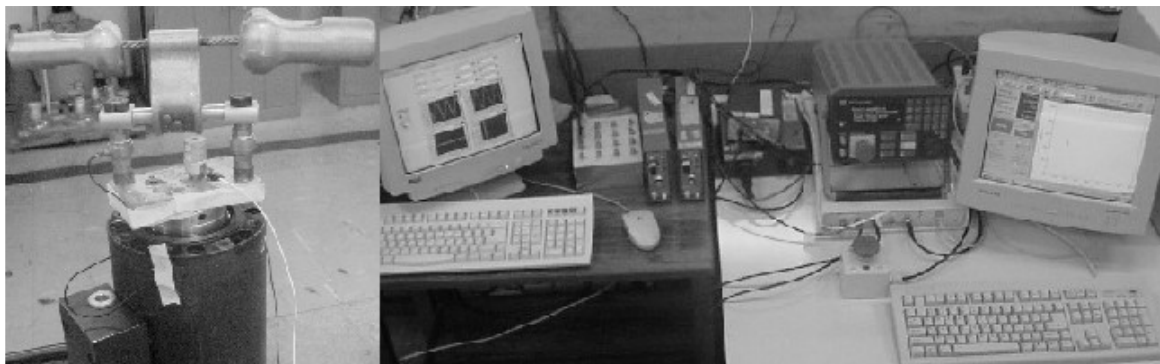
Figure 3. Experimental set-up for the frequency-response test performed with Stockbridge dampers.
