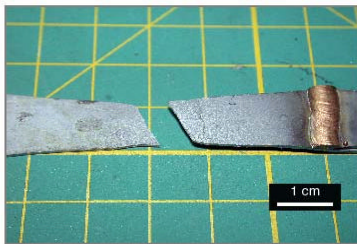
Figure 4. Detail of specimen failed in the base metal after tensile test.
