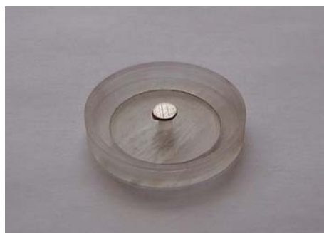
Figure 1: Sample holder with specimen used for the measurement of the amount of \alpha' martensite.
