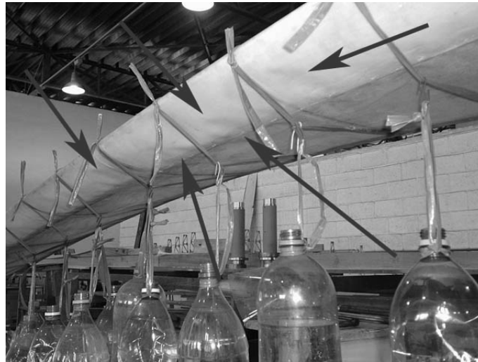
Figure 9. Local compression failure on the torsion box
