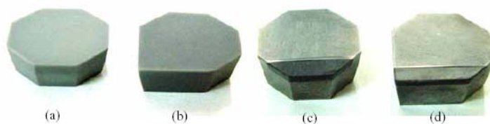
Figure 5. Tool tips used in the tests. Ceramic inserts (a) - roughing (b) - wiper. PCBN inserts (c) - roughing, (d) - wiper
