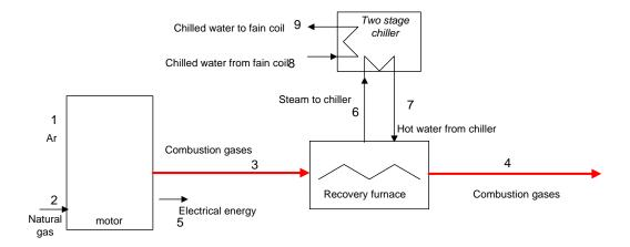
Figure 1 – Simplified diagram of the 1st configuration proposed for the shopping center under study.
