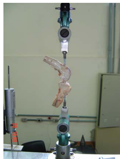
Figure 3. Gripper attached to the testing machine.
