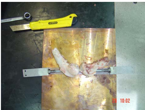
Figure 2. Gripper built with screws welded to small metallic plates.
