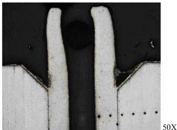
Figure 8 - Filler alloy BNi-2 applied as powder with ethyl alcohol: lack of filling and erosion of base metal
