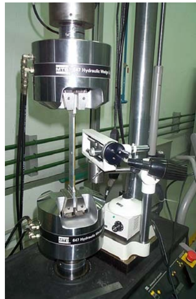
Figure 4. Coupon test in the MTS 810 device.
